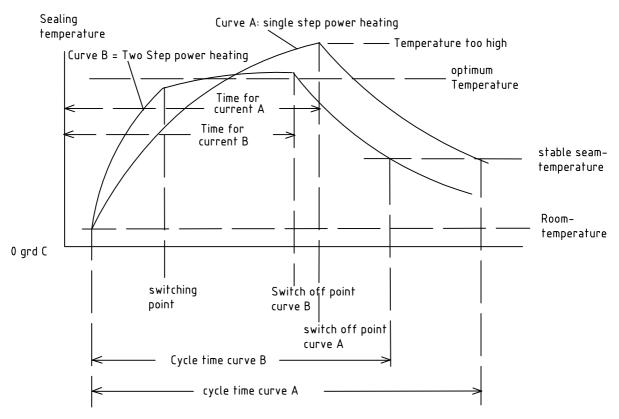
Using a patented transformer switching procedure it is possible to frequently switch on and off the welding transformer in a pulse mode without bothersome inrush currents arising.
